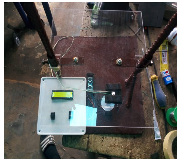
Figure 4: Constructed experimental work that determines fuel refractive index.
