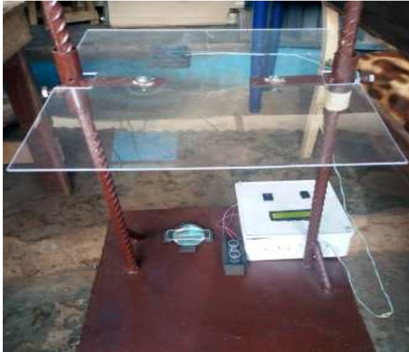
Figure 5: Side view of constructed experimental work that determines fuel refractive index
